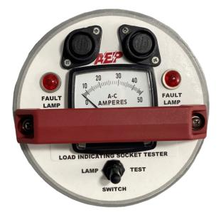
The AE Products Load Indicating Socket Tester detects the connected load inside the facility before setting the meter. This device also safely checks for phase-to-phase ground faults at the meter socket. This tester is used by meter installers to test for backfeed, load and fault conditions at the socket.
